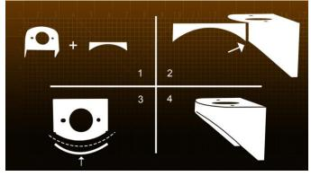
Install the new or used bushing into the bracket, and with the new or used body mount and bushing bolts and nuts, tighten the bracket into the body, for purposes of body-to-frame alignment.
