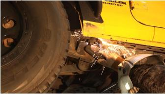
Attempt to install the part into place, and remove any debris preventing it from assembling, revealing bare metal.
