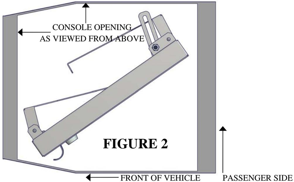
The Insert will need to rotate while being placed so that the lid/logo faces up. The fit is quite tight and may require a second effort at a slightly different angle. The Console Insert should now be resting on the bottom of the console with the logo facing up.
