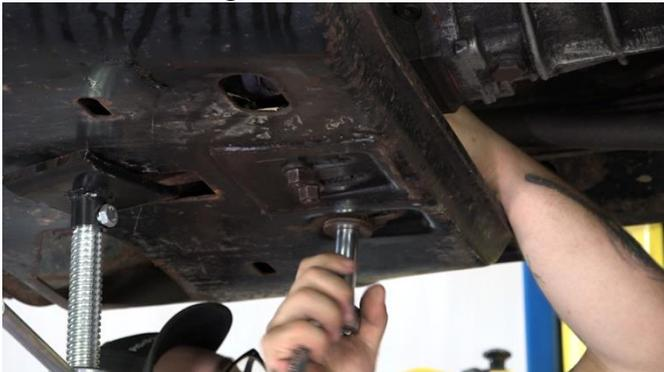
Support your skid plate with a jack or jack stand. Remove the six transfer case skid plate bolts using a 19mm socket.
