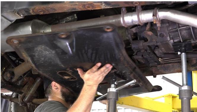
Depending on the exhaust routing, it may need to be removed or loosened to allow freedom of access to weld.
