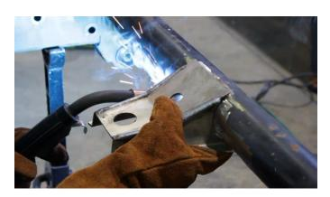
Tack weld bracket into place and test fit body bushing and bolt to check fitment.
