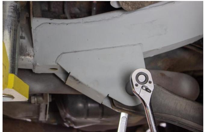
Reinstall upper control arm using 17mm socket.
