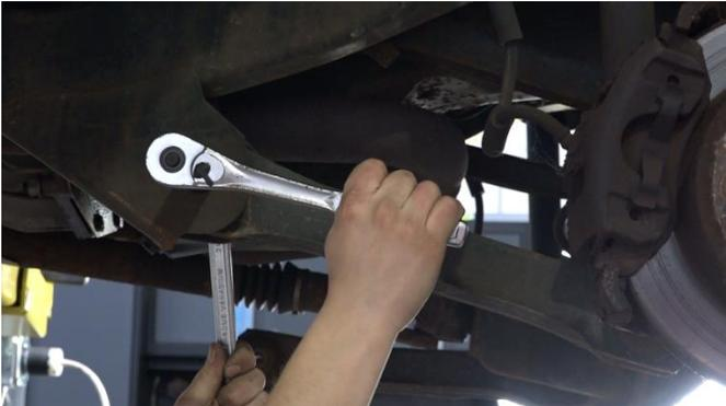
Remove upper control arm bolt from frame side bracket using 15mm socket.
