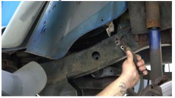
While using a tape measure, measure 1.5 inches from the top of the frame rail. Mark along the top of the frame from the front body mount bracket to the frame hole using a paint marker.
