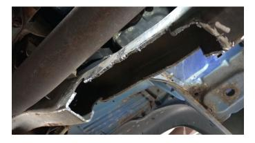
The part may fit snugly and require force. Ensure the frame rail is flush and part starts just before the front body mount for approximately 16 inches.
