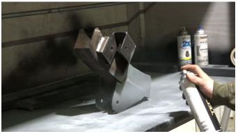
Coat the part with a weld-able primer or other rust inhibitor to help prevent or reduce the risk of rust formation.
