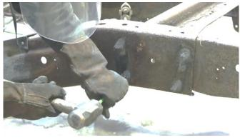
After removing your rivets, grind down the frame free of rust and debris, revealing bare metal.
