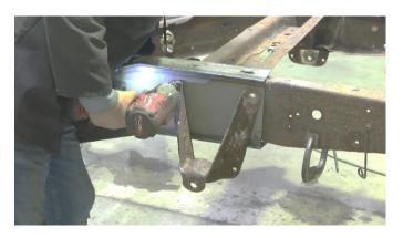
Use the remaining hardware to reinstall the end of your spare tire crossmember on the top and bottom of your frame rail.
