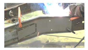
Then, clamp your plate against the frame using a cclamp, followed by welding the plate into place.
