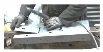
Slide your center frame section onto the frame using the frame holes to help with the alignment. Tap it into place using a hammer.
