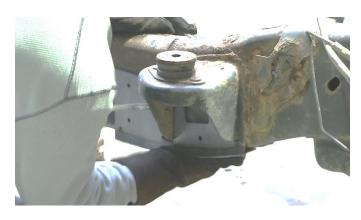
Following proper welding procedures, tac weld your front frame section into place before welding the part on fully. Weld 100% around all edges.
