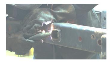
After removing your crossmember, you will need to remove a small amount of material around the perimeter of the hole you created when cutting out the factory crossmember. This will allow your replacement crossmember to slide into place. Do this on both sides of your frame rail.
