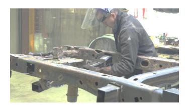
Slide the two remaining plates onto the outer side of your frame rail. Push the inner plates to where they sit against the inner side of your frame rail.
