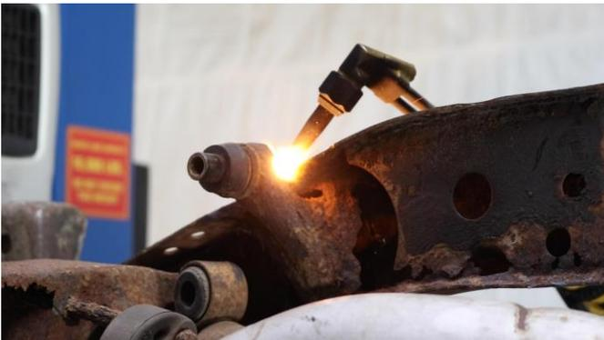
Begin cleaning the frame of any rust and debris, revealing bare metal.
