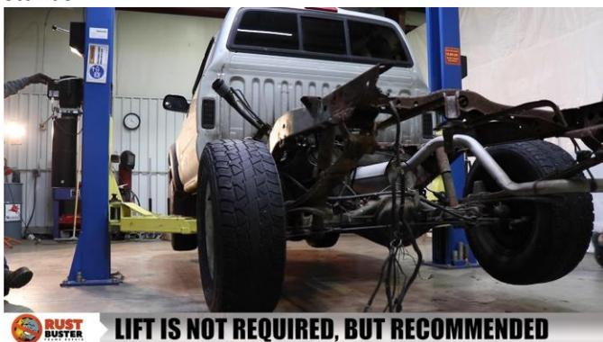
Remove your vehicle's hitch, rear bumper, and bed. For a tutorial on how to do this, please visit [www.youtube.com/rust\\_buster\\_frameworks](http://www.youtube.com/rust_buster_frameworks) for a step-by-step guide and walkthrough.
