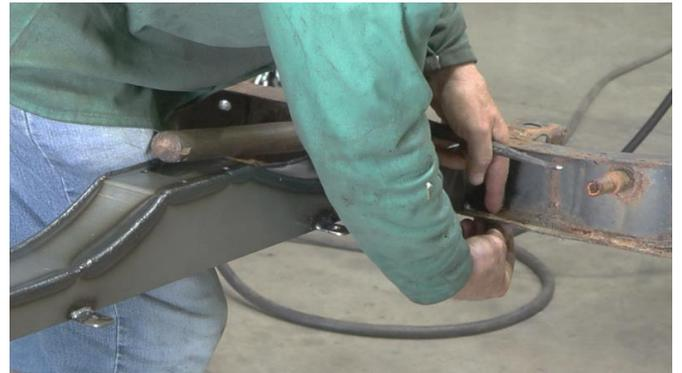
Using a 13mm socket, screw the support bars into place with the included M8 nuts and bolts.
