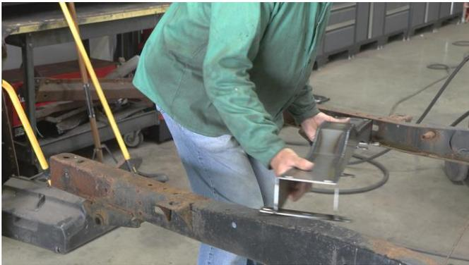
Hammer the crossmember into place, making sure the holes align.
