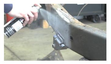
Using the silhouette where the factory body mount was originally located, hold the part up to the frame and mark off its coverage using a paint marker.
