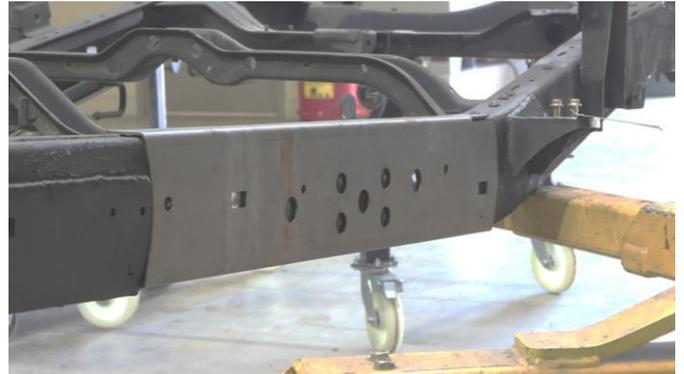
Following proper welding procedures, tack weld the center frame section onto the frame before welding the part on fully. Weld 100% around all edges.
