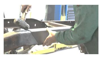
Following proper welding procedures, tac weld the over-axle frame section to the frame before welding the part on fully. Weld 100% around all edges.
