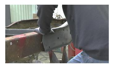
If you installed our center frame crossmember (RB7363), use a 14mm socket and 15mm wrench to install the eight bolts on the top and bottom of your frame rail to hold your crossmember and leaf spring frame section in place.
