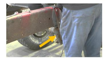
To align the leaf spring hanger with the 4WD and heavy-duty bracket, we will need to make some slight adjustments. To do this, we recommend lining up the bracket and leaf spring hangers' holes to the best of your ability. Then, using a torch, burn your way through the holes so the bolts will align properly.
