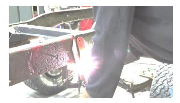
After removing the rivets, take your leaf spring bracket and screw in two of the included bolts with a 14mm socket and 15mm wrench.
