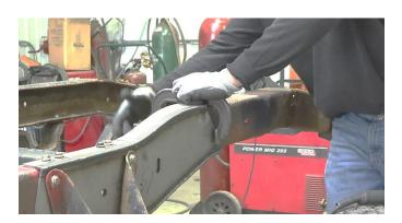
Following proper welding procedures, tac weld your leaf spring frame section onto the frame before welding it on fully. Weld 100% around all edges.
