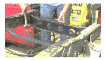
Once in place, use a 14mm socket and 15mm wrench to screw in the included M10 hardware on the top and bottom of your frame rail.
