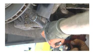
Remove your bump stop. This makes the part easier to weld on without the bump stop getting in your way.
