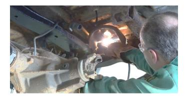
Grind down the frame free of rust and debris, revealing bare metal.
