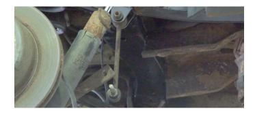
Using a 21mm socket and wrench, remove the bottom shock bolt, along with the shock. This relieves the spring so we are able to move it out of the way of our work space.
