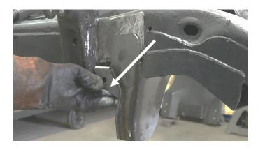
Once aligned, tac weld the support bracket to the track bar bracket before welding the parts on fully. Weld 100% around all edges.
