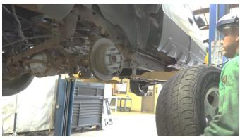
With a 21mm socket and wrench, remove the bolt securing your track bar and push it down and out of the way.
