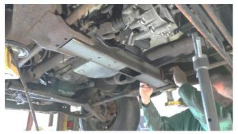
Reinstall the bolts using a 21mm and 15mm socket and wrench.
