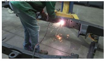
After you have cleaned the appropriate areas of the frame, paint the work area with a weld through primer. This will help prevent rust development, protecting against water, salt, and other road debris.
