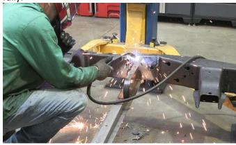
After you have finished with the first side, you may move to the opposite and begin the same process. Make sure to weld 100% around all edges to ensure that the part is completely secured to the frame rails. Holes in the weld can allow for water and other debris to enter the space and corrode the adjoined components.
