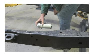
Additionally, the primer will set the base on which the crossmember can be sufficiently welded.
