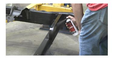
Although our parts do ship with an oil coat to prevent oxidation, we recommend applying our Rust Buster Rust Converter & Primer Spray Paint (RB9917) for additional protection.
