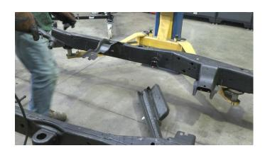
After you have successfully removed the OEM Front Frame Support Crossmember, use your hand grinder to clean the areas of the frame where the crossmember was previously attached. Remove all rust possible, as you will need to create a smooth and clean point at which you can attach your replacement crossmember.
