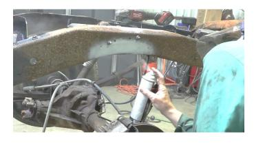
Our part features a perforated plate that can be removed to fit over your existing bolts. If you decide not to remove the bolts, cut out the perforated plates on the top and bottom of your frame section.
