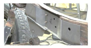
Hold the fuel tank bracket up to the frame and using a 15mm socket, screw the 4 nuts into place.
