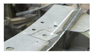
Then, we'll need to bend over the top section so we can slide our part onto the frame. Cut one side of the top section and bend it over with pliers.
