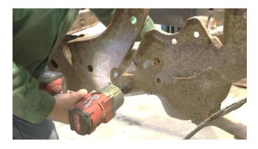
With an 18mm socket, remove the bolt retaining the leaf spring.
