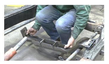
Using a 15mm socket, install the two bolts and nuts on each side of the crossmember.
