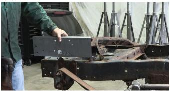
Our part features removable/perforated plates to allow the part to go around the spare tire crossmember's retaining rivets. If you are not replacing the crossmember, remove these plates as needed.
