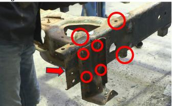
**NOTE**: We only include hardware to install your new spare tire crossmember. We do not supply additional hardware to resecure your leaf spring hanger. If you wish to reinstall your factory hanger, you will need to either supply additional M10 hardware, or purchase and install **Rust Buster's RB7801L/RB7801R Rear Frame Sections**.
