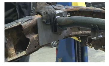
Tac weld the pre-welded side into place and verify its alignment. Align the opposite side's plate with the top of the frame rail and tac weld it into place.
