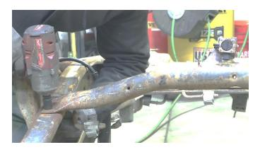
Then, cut out the rivets. You can punch out the rivets using a punch.
