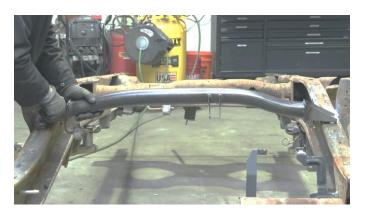
Once you have your crossmember in place, take the included hardware and screw them into place where your rivets were originally located. Then, tighten your hardware with a 14mm socket and 15mm wrench.
