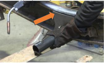
Tac weld the part into place and verify its alignment.
