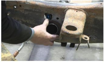
Completely weld the plate around the outside in inner edges.
