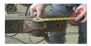
Using the measurements you took on the opposite side of the frame, mark where the center will be with a paint marker.
