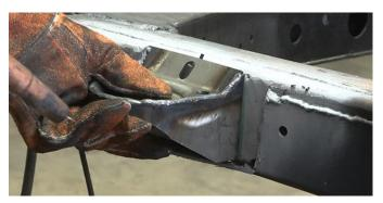
Remove any potential fire hazards from the work area. Following proper welding procedures, tack weld the part onto the frame before welding the part on fully. Weld 100% around all edges.
