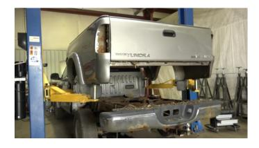
Hold the part up to the frame and take note of its coverage. Mark out your cleaning and grinding area.
