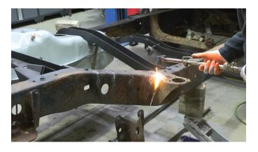
Grind away any remaining rust and debris revealing bare metal. Coat the part and work area with a weld-through primer to help prevent against further rust development.
