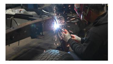
Reattach your leaf spring hanger and body mount bracket. The original holes that the leaf spring rivets came out of are going to be higher than the parts holes. This is because of the added material to the outside and bottom of the frame. You must take a die grinder or drill bit to the frame holes to match the holes on the part.
