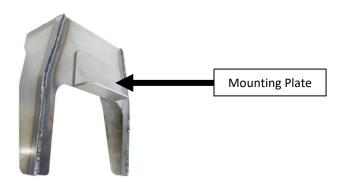
Following proper welding procedures, tac weld your plate to the back of your rear cab mount.
